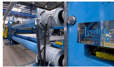
Thrive e-Drive® Leveling System - After many years of success with our e-Drive® leveler, our innovation continues with the development of Thrive, our 3-drive precision leveling platform. The Thrive system features increased material stress reduction and makes corrections automatically using laser artificial intelligence technology.
