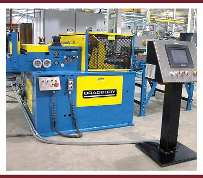
With its state-of-the-art features, the B.O.S.S.™ provides high production rates with close tolerance shearing. As an added feature, the shear can be equipped with notching or slitting - allowing the B.O.S.S.™ to work in various applications. The intelligent drive and shear system allows the B.O.S.S.™ to be close-coupled to a new or existing roll former. The unique orbital design provides fast, smooth production rates, and the acceleration or deceleration of the line does not affect the cut.
