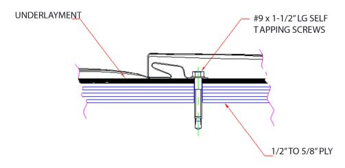
Side view elevation of the hidden fastening concept showing front and back clips.
