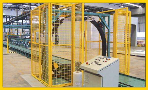
Our new Stretch Wrapper and Conveyor System is ideally suited to panel stacking applications and offers enhanced flexibility for wrapping short stacks.
