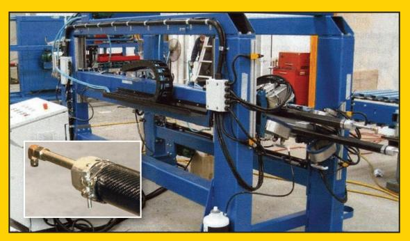
Our new Low-Pressure, Self-Cleaning Spray Glue System can be tailored to most Laminated Sandwich Panel Lines – regardless of manufacturer. Unique design delivers a precise component mix of 2 Part Polyurethane Adhesive in a variable volume range from 240 grams/minute to 1,540 grams/minute. Spray heads are operator adjustable and can be customized for panel line fit and tight clearances.
