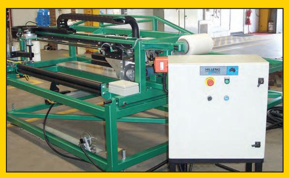
The Film Insertion Unit is an optional part of the Hilleng Deep Profile Laminating System that installs between the Deep Profile Uncoiling Unit and the Deep Profile Rollforming Unit at the head of the laminating line. It is designed to facilitate removal of unwanted core material to allow an overlapping joint needed to join the ends of mating Deep Profile Roof Panels. The unit applies a protective film to the roof panel steel skin which prevents the core material from bonding to the skin.
