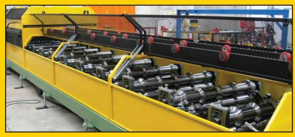
The Deep Profile Roof Rollforming & Decoiling Unit is used to laminate Deep Profile Roofing Panels in 3 rib, 4 rib, or 5 rib styles. Located at the start of the Hilleng Panel Laminating Line, the unit continuously feeds coil steel into its rollforming section to form the ribbed profile. The rollformed sheet is then fed into the lead-in section of our Hilleng Main Press, where adhesive is applied to the underside steel skin before it is laminated to the core insulating material.
