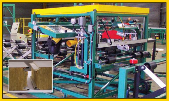
The upgraded and fully automated Coldwire Unit uses an abrasive wire band to cut through core insulating materials, including Mineral Wool, PU, PIR, XPS, EPS or Phenoelic Panels. The unit is located after the Cut-Off Unit and linked to the Main Control Console. Photoelectric sensors and servo drives initiate the cutting cycle as the panels move through the unit.
