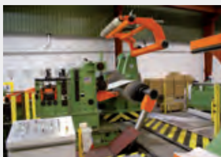
Mobile Tension Unit with recoiling angle and Strip Tension Control
