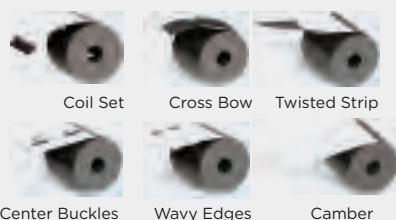
Leveling defects corrected with Athader's Levelers.
