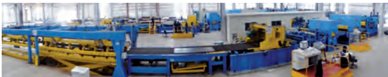
Heavy Gauge Cut-To-Length Line with Flying Shear and Double Station Drop Stacker
