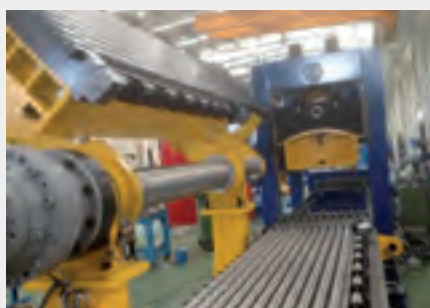
Leveling Cartridge with "Book Opening" System for easy maintenance and cleaning
