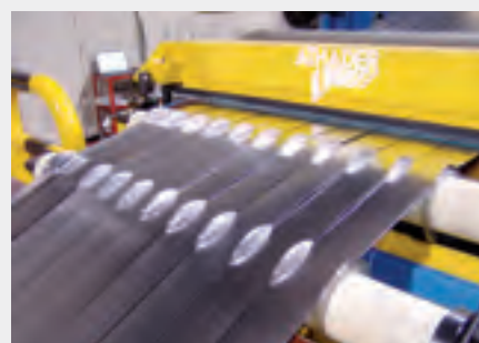
Dual Separator shaft for the optimal guiding of strips
