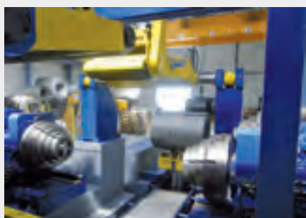
Double Stepped Uncoiler with Electric and Automatic Back Tension
