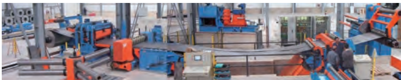
Medium Gauge Slitting Line running in pull assist mode
