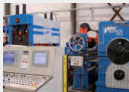
Precision Leveler & Rotary Shear, with Pre-setting and Automatic Line Adjustment.
