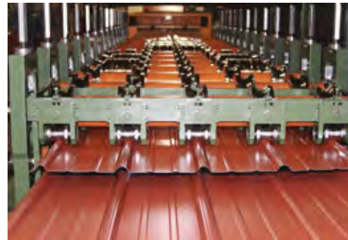
Through-fastened panel exiting Bradbury roll former.
